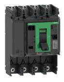
Circuit breaker basic frame, ComPacT NSX400H, 70kA/ 415VAC, 4 poles, 400A frame rating, without trip unit
